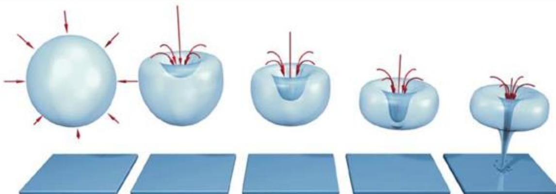
Figure 2 Micro-jet creation through collapsing cavitation bubbles (<http://eswt.net/cavitation>)
