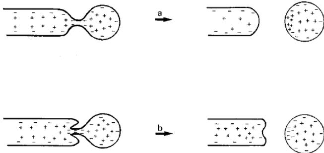
Figure 3 Build-up of large charge differences as a water droplet breaks away from the jet within a cavitation bubble (LePoint, De Pauw et al. 1997)
