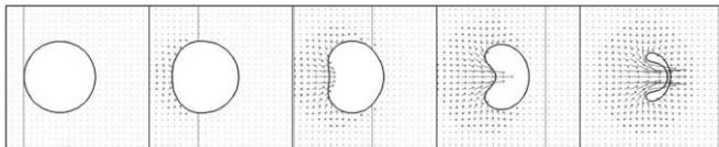
Figure 13 Simulation result of the interaction of a pressure pulse of 0.528 GPa with a bubble of radius 1.0 mm (Ohl, Klaseboer et al. 2015).
