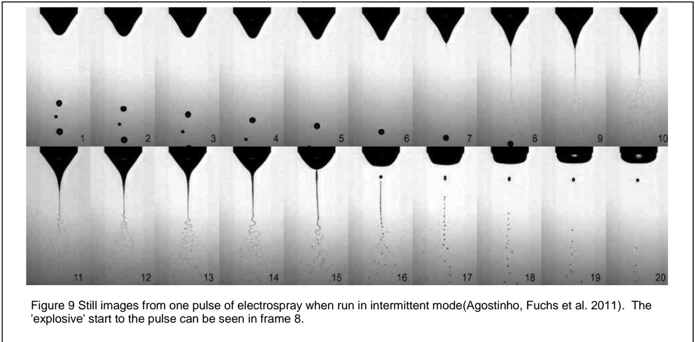
Figure 9 Still images from one pulse of electro spray when run in intermittent mode (Agostinho, Fuchs et al. 2011). The 'explosive' start to the pulse can be seen in frame 8.
