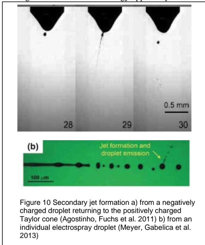
Figure 10 Secondary jet formation a) from a negatively charged droplet returning to the positively charged Taylor cone (Agostinho, Fuchs et al. 2011) b) from an individual electro spray droplet (Meyer, Gabelica et al. 2013)
