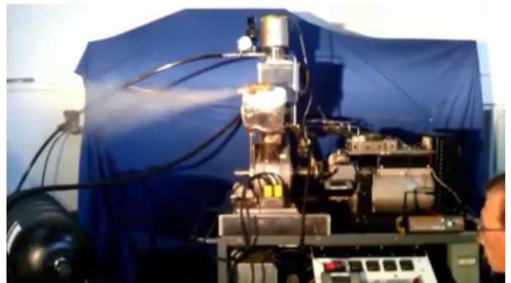
Figure 15 Stills from video of CES steam generator. A) shows the appearance before steam has emerged. B) shows the situation as the steam emerges. The steam in fully vapour and as such is invisible, but its presence is clear from the refraction of light from objects behind the steam. c) The steam cools and the water vapour condenses out into visible droplets.
